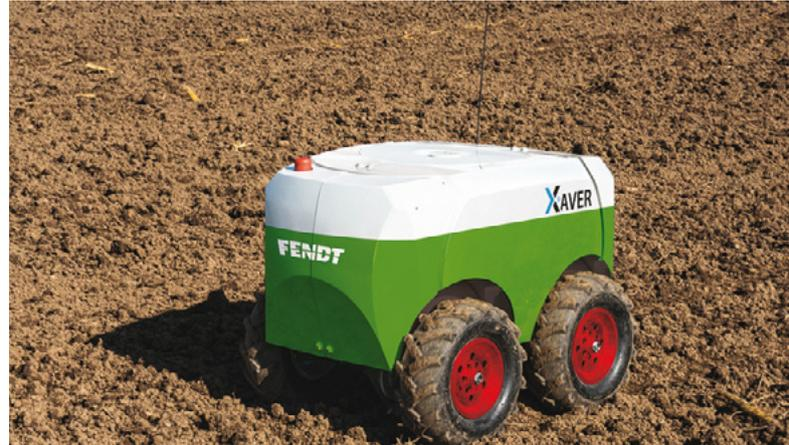
Fendt's new Xaver system uses small robot units operating in swarms and a cloud solution to plan, monitor and accurately document the precise planting of corn.
