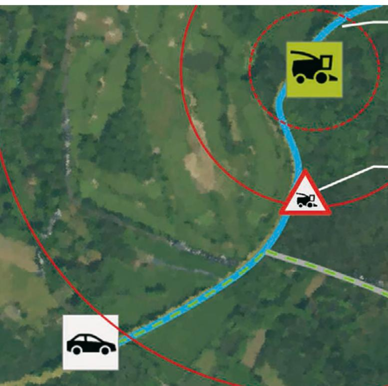
**The location of an agricultural machine is transmitted from the telemetry data to the navigation systems of cars and trucks in 'real time'.**
