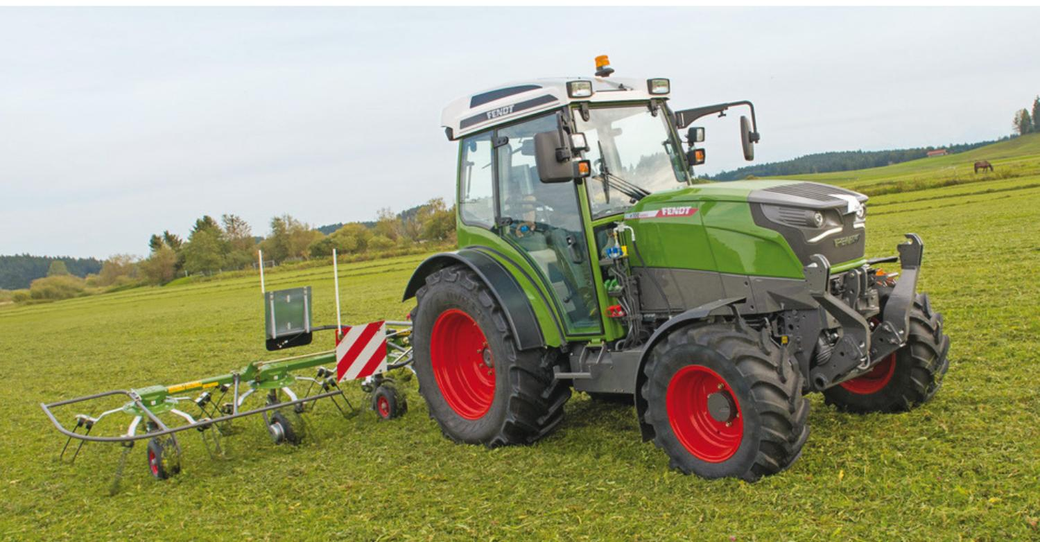
**Fendt's e100 Vario, an all-electric compact tractor with 50 kW power output and winner of the DLG silver medal at Agritechnica.**
