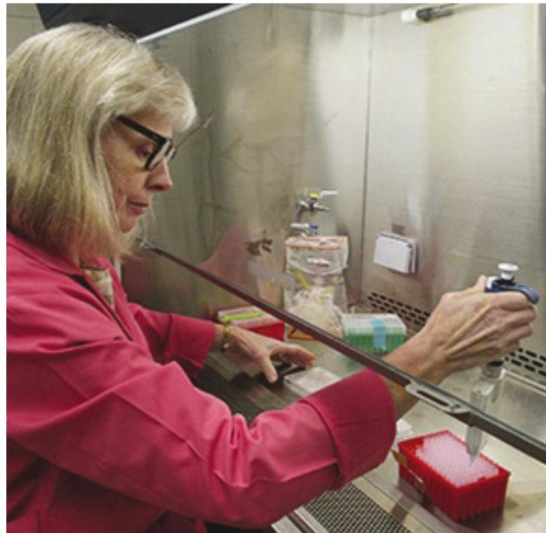
Chemical engineer Pat Slininger adds a specialty sugar called isomelezitose to bacteria to test the sugar's cell-protecting properties. (PHOTO: Chris Skory)
